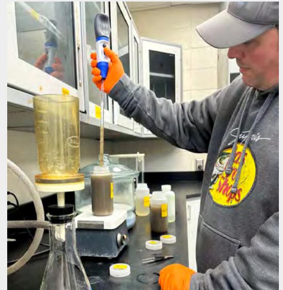
Pictured: Wastewater Supervisor Kevin Hudson completes daily suspended solids testing. This test helps determine if the wastewater treatment plant is operating effectively, and operators are able to make adjustments in the treatment process based on sample results.
